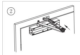
1-Insert the adjusting rod into the folding arm.
