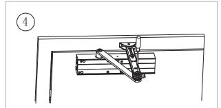
Open the door to the desired stop angle, ensuring that the teeth on the adjustment plate engage correctly with the teeth on the main arm bracket (to prevent slipping), and then tighten the toothed screw with an internal Phillips screwdriver.
