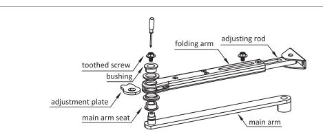
The positioning angle is factory-set between 90° and 100°. If you need to set the positioning angle, first loosen the toothed screw, then fix the door at the desired stop angle, and finally tighten the toothed screw.
